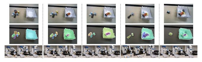
Fig. 6. Setup for top-down grasping with segmentation. Robot images on each column show the three stages: approach, pickup and placing in the bin.
